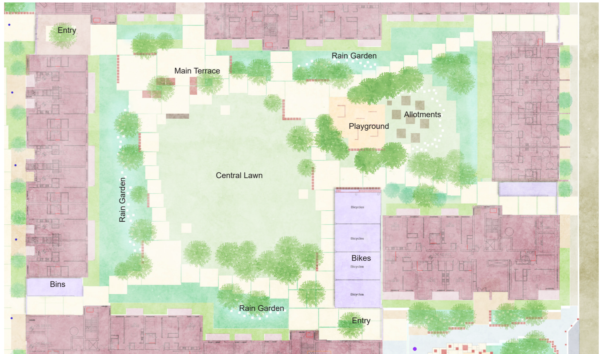
Plan of Large Courtyard showing the key features of the proposed design
